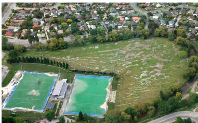
The Porritt Park hockey fields were damaged by both liquefaction and ground surface undulations. Remaining evidence includes pooling water and sand in the open field to the right of the hockey fields.
